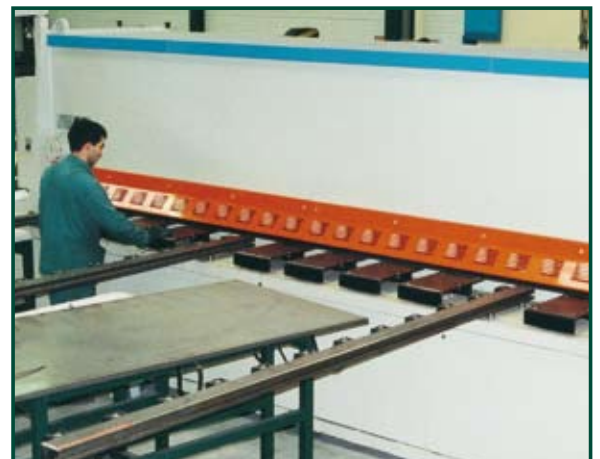
Shear cutting, angle notching, bending.
